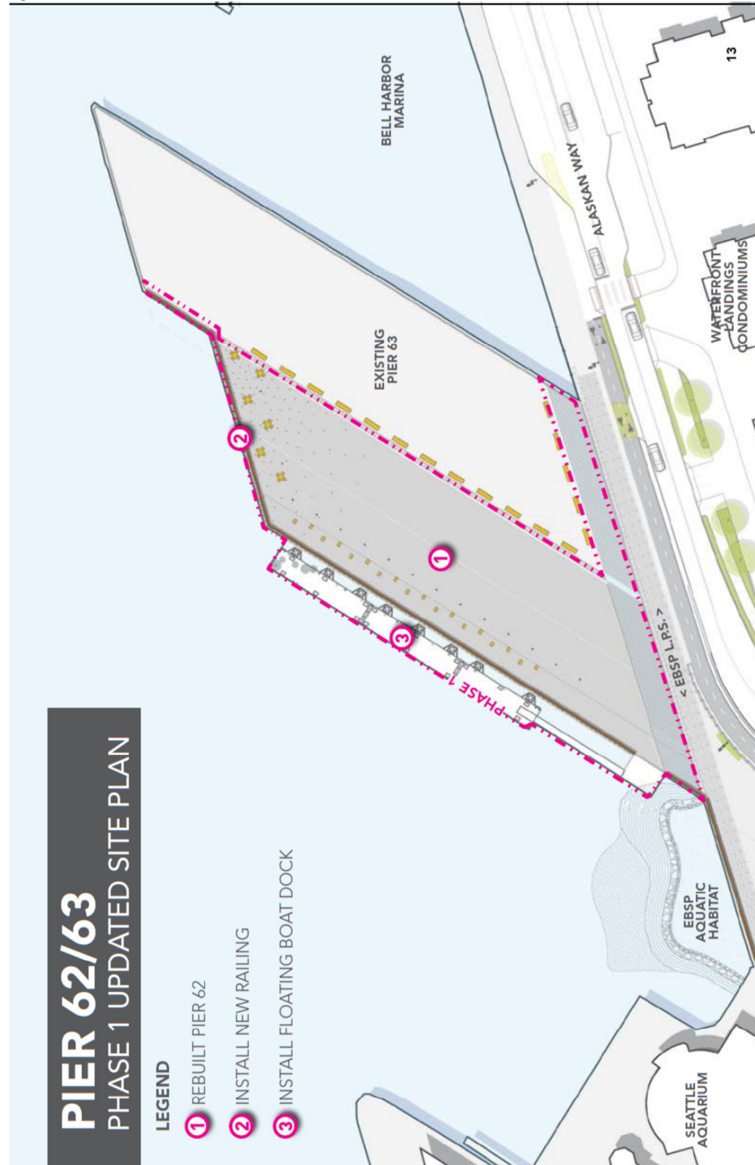
Figure 4: Pier 62/63 Phase 1 Rebuild Plans
